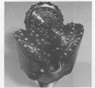
TYPICAL ROLLERCONE drill bit, basically unchanged since its invention in 1908 by Howard Hughes, Sr. Cones with tungsten inserts revolve as bit head rotates.
